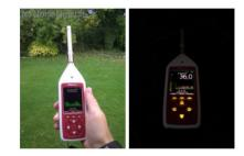
Most environmental noise surveys demand the use of a Class 1 Sound Level Meter that can make repeating measurements, such as the 5 minute LAeq and L90 (background noise).
